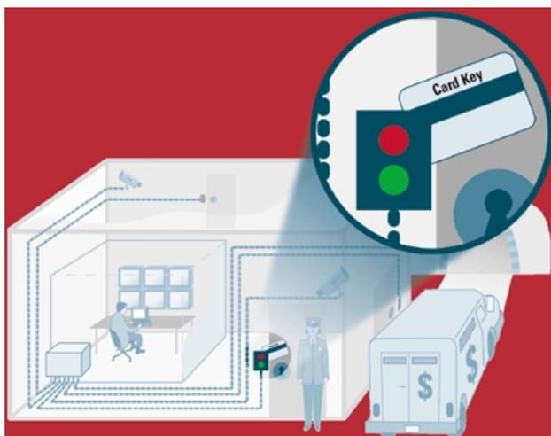
Access Control Servers function like door access cards and the gatekeeper that oversees site security, providing centralized authorization, authentication and accounting (AAA) for traffic and users.
